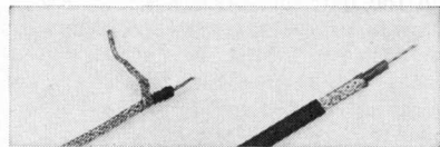
Examples of shielded wire and coaxial cable. The wire (left) is the type with a single inner conductor. Multi-wire cable of similar construction is often used. The coaxial cable shown (right) is a small type (RG-58/U). Cable of this general construction is available in several different diameters, for handling various power levels.
