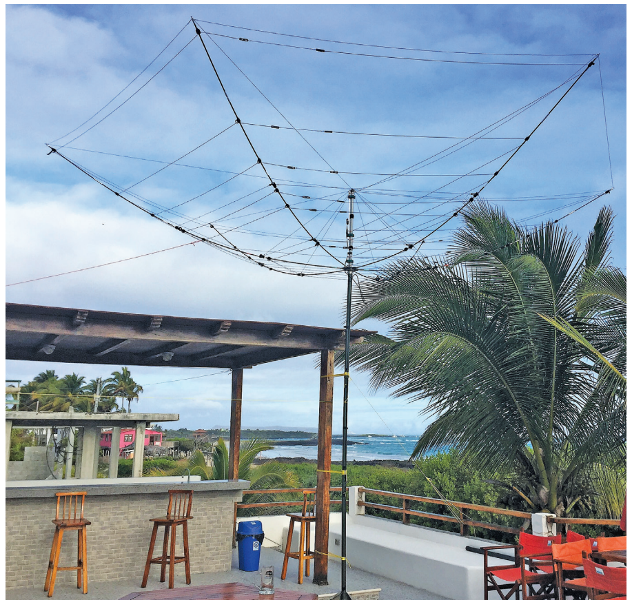
The hexagonal beam antenna that was used for the HD8M operation on Isabela Island. [Jim Millner, WB2REM, photo]
